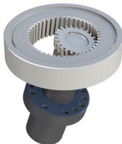
Figure 1: Gear skiving of internal and external gears with a relation of tool and workpiece axis arranged at an angle to each other
