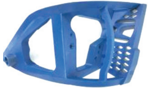
The lighter, more ergonomic 3D printed taillight inspection fixture.
