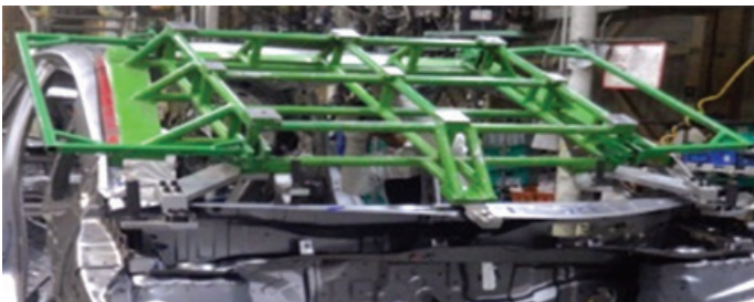
The heavy, conventional windshield inspection jig.
