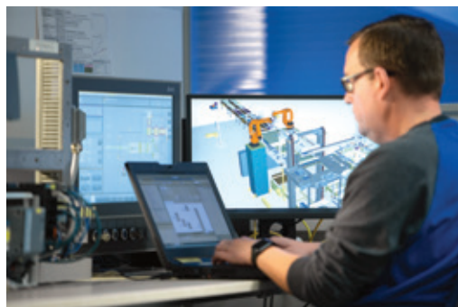
When all data is provided through a shared interface, machines can be quickly and efficiently commissioned on screen.
