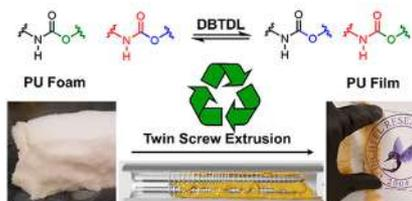
**Researchers from the University of Minnesota and Northwestern University have improved the recycling process of polyurethane through the development of a twin-screw extrusion process that improved mixing and air removal in foams.** *Credit: Sheppard et al., ACS Central Science*
