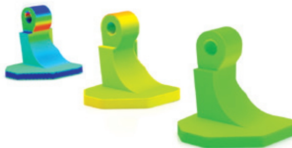
Three phases of automated optimisation show compensation for distortion using the Metal Binder Jetting module in Simufact Additive. The results show the deviation between the simulated part and its initial CAD geometry – blue / red: bad; green: good.
