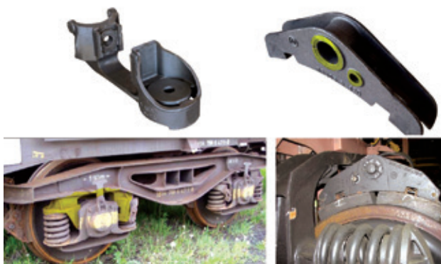
Examples of rail components which can be machined with Dormer Pramet's standard indexable milling tools.
