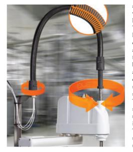
and the fixed end, as well as the corrugated hose with the e-rib. The special feature lies in the new rotary connection, which absorbs the torsional forces. Here, integrated ball bearings ensure a smooth-running energy supply system that is resistant even to high accelerations. The corrugated hose is reinforced with an e-rib so that it can only move in one spatial direction. The guide elements on the sides give the hose unsupported length.
