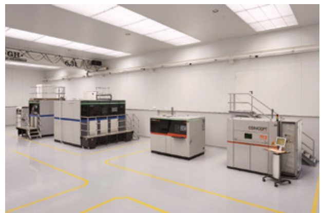
GE Additive Concept Laser M Line system installed at EROFIO Group's facility next to a GE Additive Concept Laser M2
