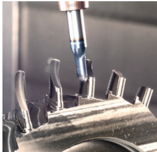
Fig. 4 – Trochoidal rough milling of a blisk airfoil by a multi-flute solid carbide endmill, which is mounted in a heat shrink chuck.
